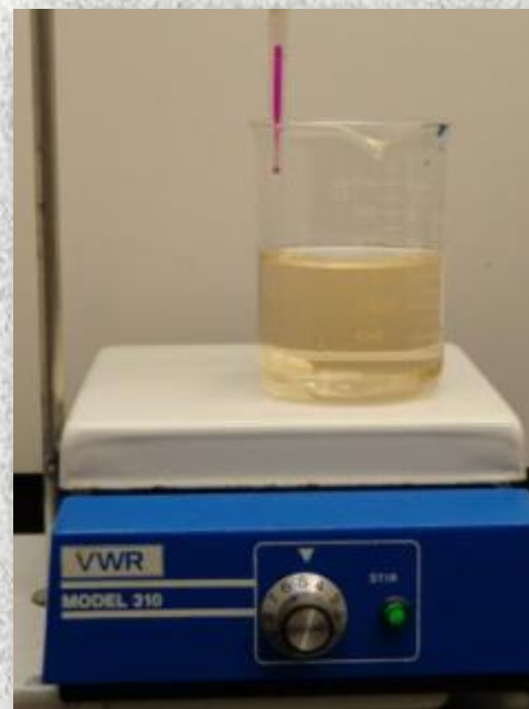
Cider juice at start of titration (blue) and at final point (yellow)
