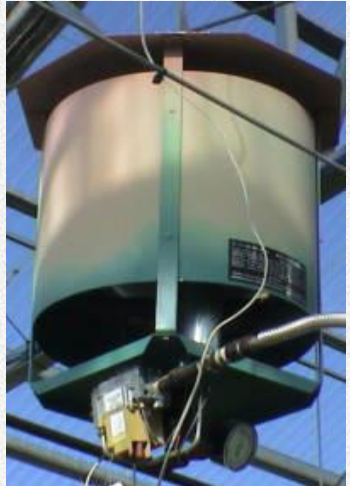
CO 2 generator based on combustion of natural gas
