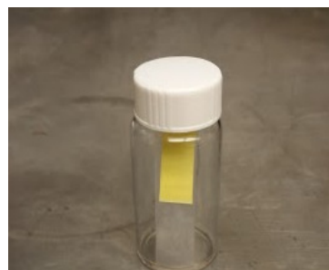
Amygdalin (0-100 \mu\text{g} ) + 50 \mu\text{L} of 3U/mL \beta -glucosidase enzymes in pH 8 phosphate buffer + picrate paper
